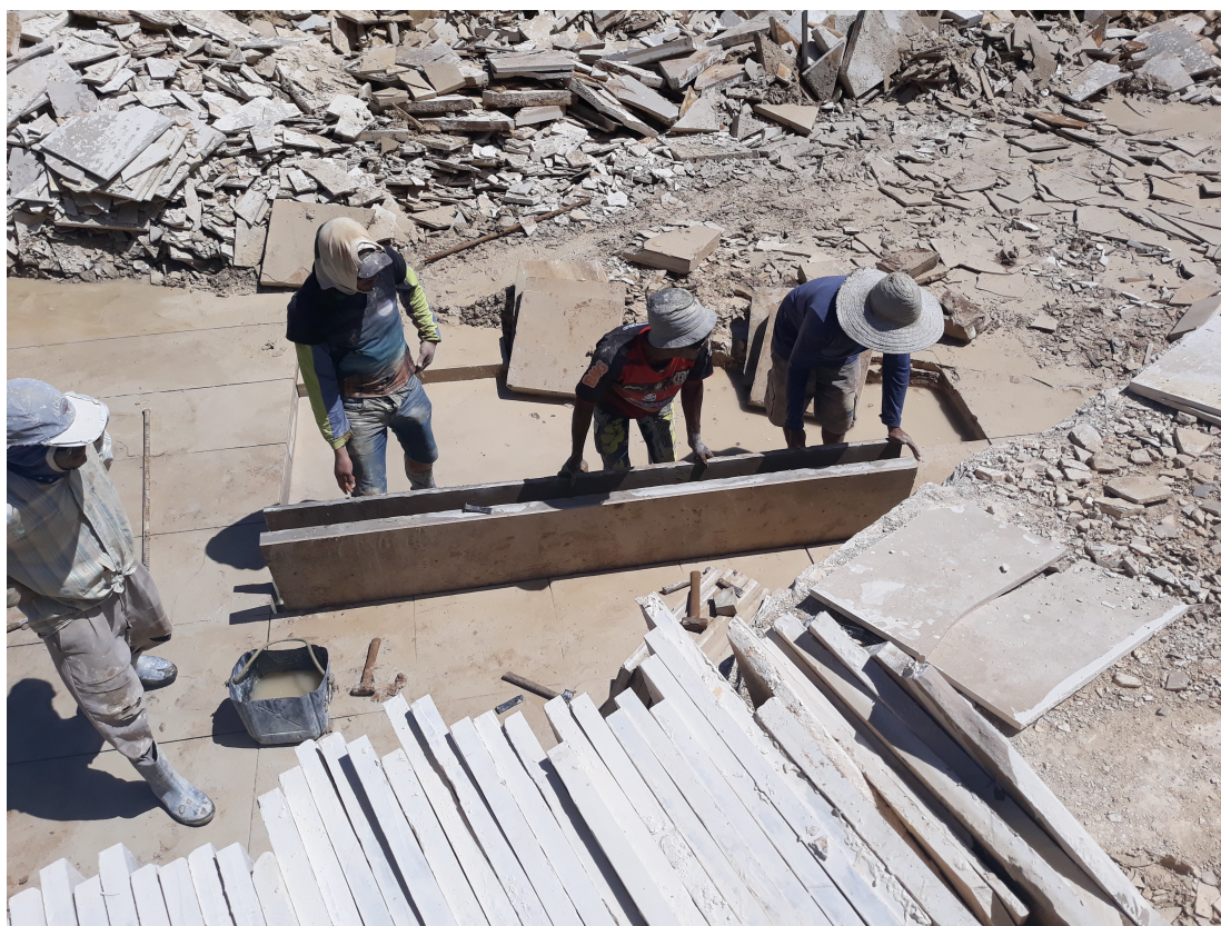
Figure 5 – Manual separation of blocks for limestone production.
