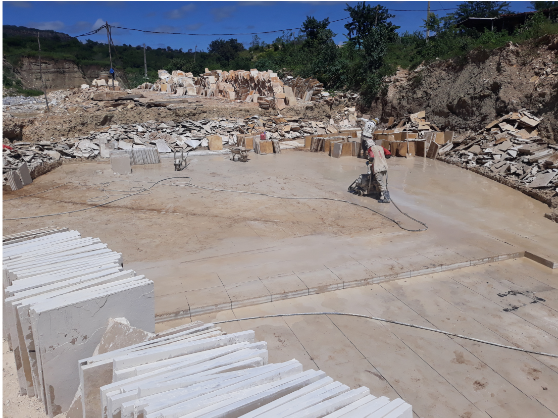
Figure 4 – Mining front of limestone as executed currently. The high ambient temperature, landslides, and electric shock are the main risks underlying operators activity.
